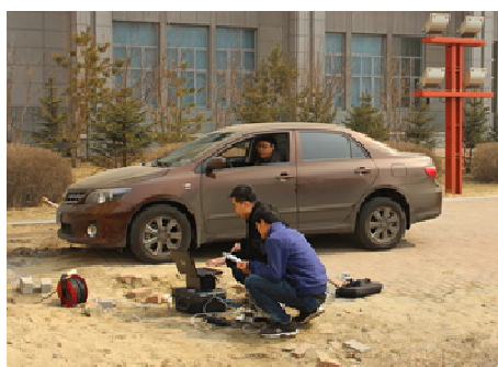
图 12 A 场地小汽车现场动态加载-卸载试验 Fig.12 Car dynamic loading-unloading test on site A
